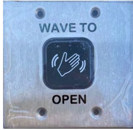
Image description: Image of the Premium Magic Switch MS41-D Touchless Actuator button, with the words “wave to open.”
