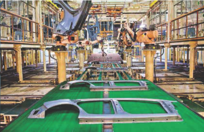
Robots with suction cups position body panels on inventory racks.
